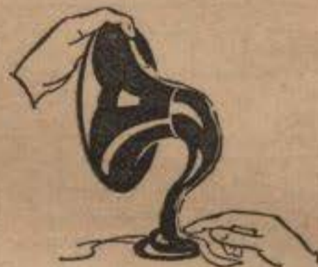
If the LISSENOLA Horn were straightened out it would measure 28 inches. This length of horn enables the sound waves to flatten out gradually and so prevents distortion.
